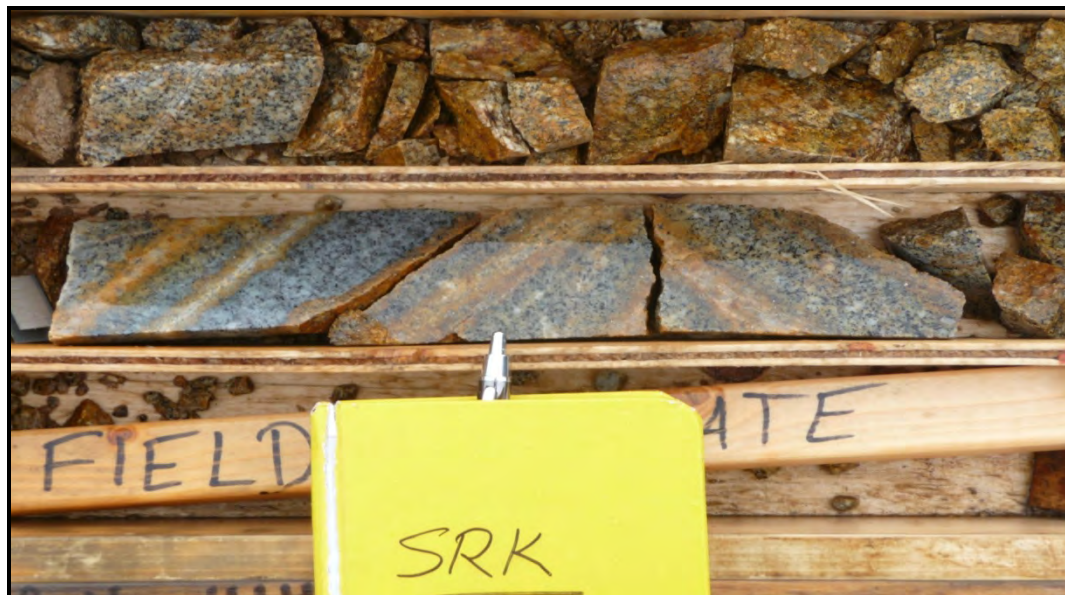
Figure 12.2 Photograph of Core with Strongly Oxidized Quartz Veins and Veinlets within Fresh Granodiorite Core
