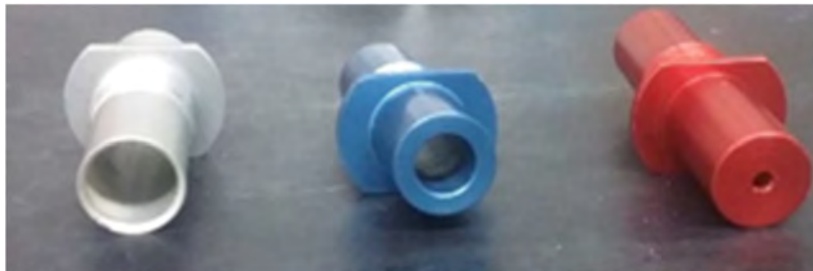
Figure 3-2: Inlet Jet Sizes: TSP (grey), PM 10 (blue), and PM 2.5 (red)
