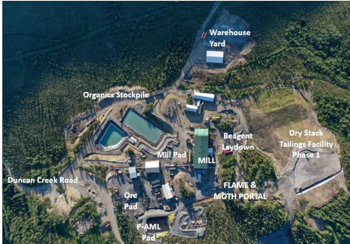
Figure 2-2: Mill and Warehouse Yard Footprint (2022)
