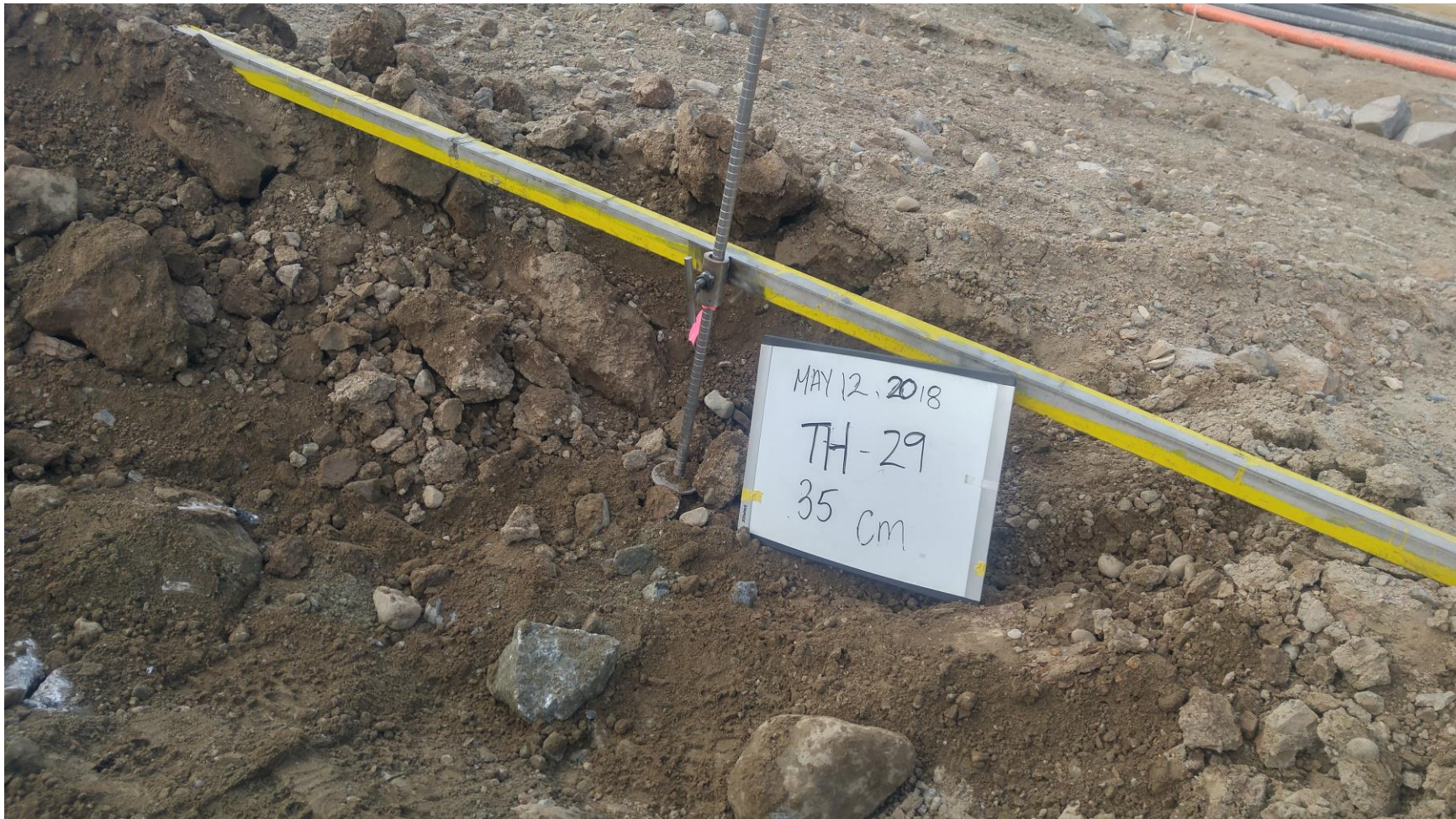
Figure 16-4: Test Pit TH-29 Measurement May 12, 2018 (0.35m depth)
