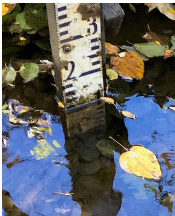
Figure A-12 Staff Gauge at W1
