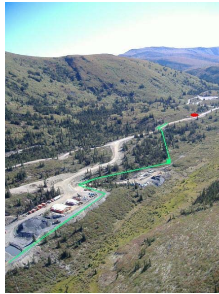
Picture 3.2. Sump water pipeline and discharge route (green line) to bladder (green square) and receiving end point at Wedge Pond (red circle)
