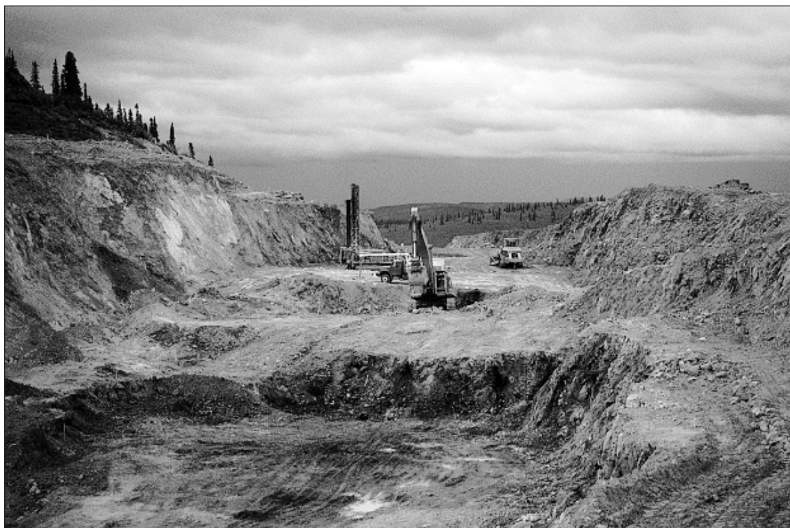
Figure 7. Brown-McDade open pit at BYG Natural Resources, Mt. Nansen Mine. The upper oxidized portion of the vein system is currently being mined.
