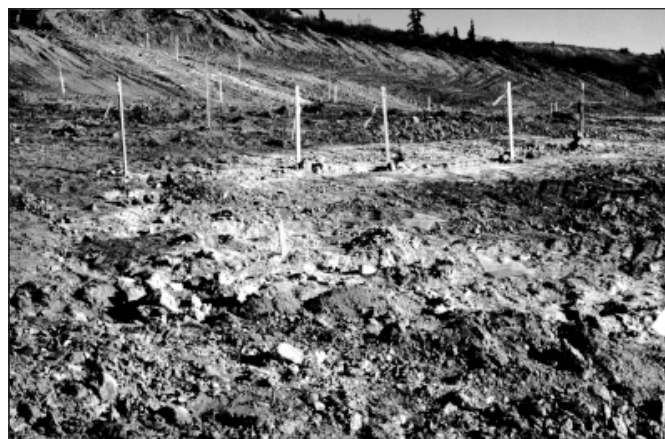
Figure 3. Part of the stripped Flex zone, showing drag-folded main vein with an envelope of bleached white clay. Looking southeast from section 3+10 N. The standing pickets are about one metre high.
