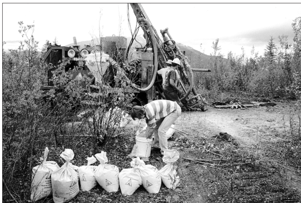
Figure 35. Midnight Sun Drilling of Whitehorse performed reverse-circulation drilling on the Wayne property of Eagle Plains and Miner River Resources. Viceroy Resource Corporation optioned the property and conducted trenching late in 1997 and plans on further drilling in 1998.
